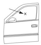
3. With the tip of a key, tap the center of the driver's door window.
